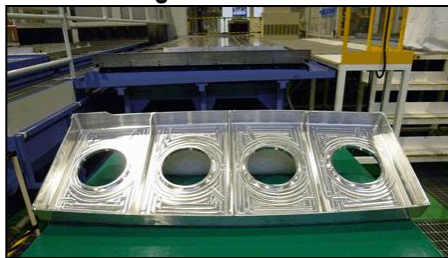
First metal cut for the MRJ's horizontal stabilizer ©Mitsubishi Corporation
